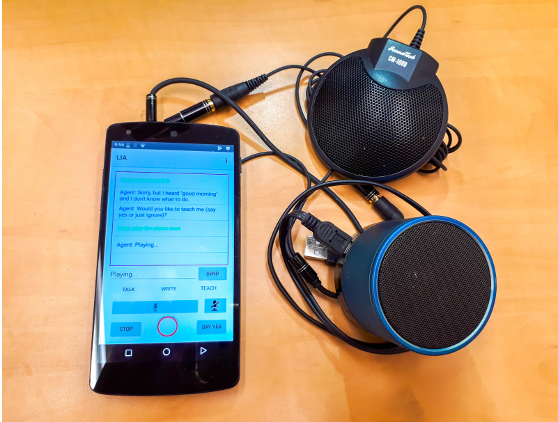
Figure 1: A photograph of LIA connected to the microphone and speaker.
