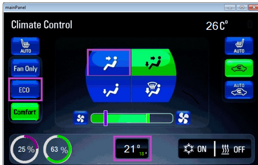
Figure 2.2: A screen-shot of the GUI with CARE's advice. In this example, the driver set the temperature to 18°C (rather than 21°C as advised by CARE), the fan to 4 (rather than 1 - as indicated by the purple line), the air delivery to face and feet (rather than face-only) and the mode to "comfort" (rather than "eco"). This resulted in an energy consumption level of 63% of the maximal energy consumption level (right green circle), rather than only 25% if the driver would have followed CARE's advice (left purple circle).
